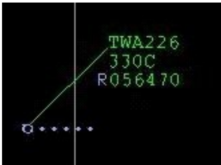
Figure 3. Example EARL GCNSS Display ADS Aircraft Logged in Not Under Control
