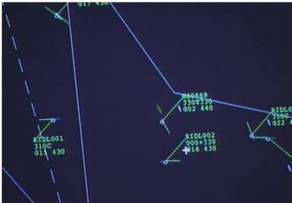
Figure 3. Example EARL GCNSS Display ADS Aircraft Logged in Not Under Control
