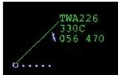
Figure 3. Example EARL GCNSS Display ADS Aircraft Logged in Not Under Control
