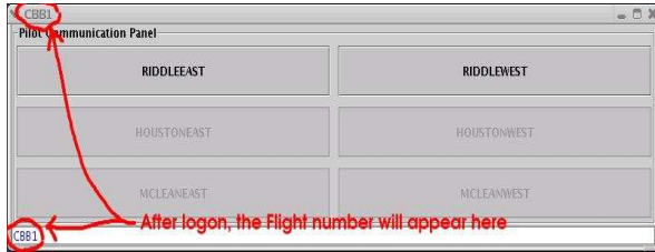
Figure 6. Aircraft, CBB1, logged onto the pilot VCS system
